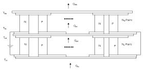
Fig. 1 Schematic diagram of the double stage TEC
